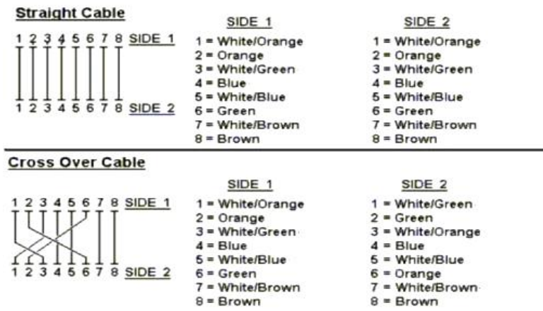
Figure 4: Straight-Through and Crossover Cable
